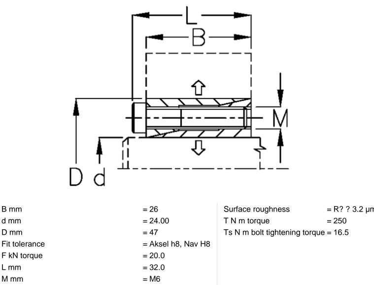
P N/mm2 surface pressure on shaft/hub = 75
